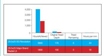
The SG Revolution tyres achieved over double the working hours of a machine fitted with a major brand radial tyre.
