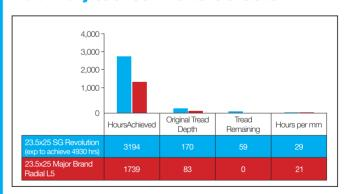
In a transfer station a JCB loading shovel achieved over 83% more hours working with SG Revolution tyres fitted.
